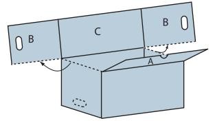
4 Fold both B panels over the center of panel C.
