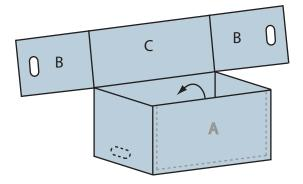
5 Fold panels B and C into carton. Open B panels up inside as shown. Panel C will make up the bottom of the carton.
